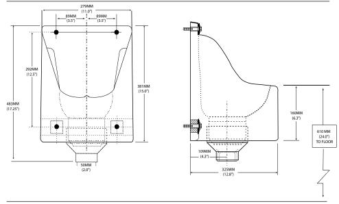
**CODES/STANDARDS APPLICABLE:** Complies with ANSI Z124.9 and ASME A112.19.19. Corresponding DOD Standard: Z124.9-D2D4X2X1.
